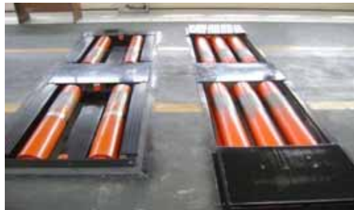
Gambar 4.10. Spedometer Tester Sumber : Dishubkominfo Kabupaten Sleman
